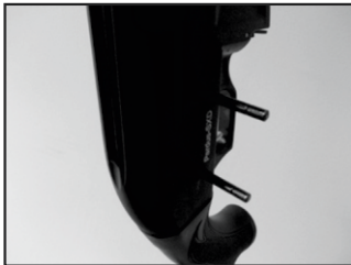
7. PUSH THE TRIGGER GROUP PINS AND TAKE THEM OFF.
