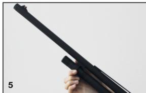
Hold the barrel ahead of the guide ring and slide the barrel into the receiver. DON'T FORCE IT! ( Photo 5 )
