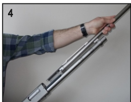
Hold the barrel ahead of the guide ring. Slide the barrel guide ring over the magazine tube into the receiver. (Photo 4) DON'T FORCE IT!
