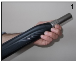
Remove the magazine cap. (Photo 1)
