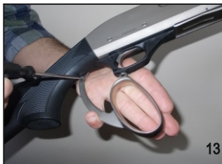
Unscrew the connector screw of two rods of mechanism and lever. (Photo 13)
