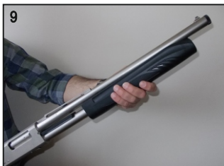
Remove the fore-end. (Photo 9)
