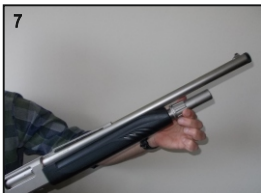
Screw the magazine cap. (Photo 7)
