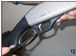
Unscrew the connector screw of lever from the trigger guard. (Photo 12)
