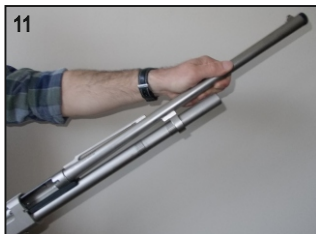
Slide the barrel guide ring over the magazine tube and take out. (Photo 11)
