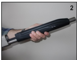
Remove the fore-end. (Photo 2)
