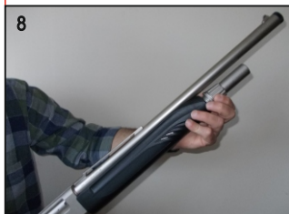
Remove the magazine cap. (Photo 8)
