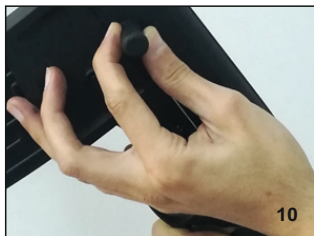
Bolt handle is screwed into the handle bracket for left-hand users ( Photo 10 )
