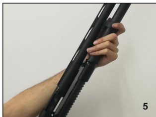
Hold the barrel ahead of the guide ring and slide the barrel into the receiver. DON'T FORCE IT! ( Photo 5 )
