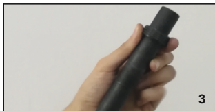
Unscrew the barrel locker nut (Photo 3)
