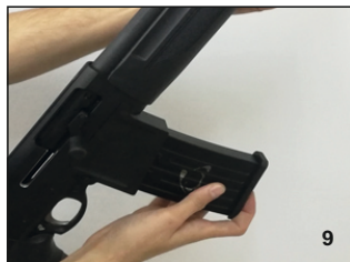
Insert the magazine and shotgun is ready for use ( Photo 9 )
