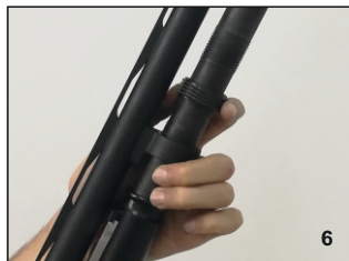
Screw on the barrel locker nut ( Photo 6 )
